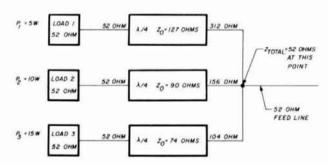
fig. 7. By selecting the impedance of the matching sections, an unequal power division can be obtained. This procedure is useful when trying to create a particular radiation pattern from a group of antennas.
